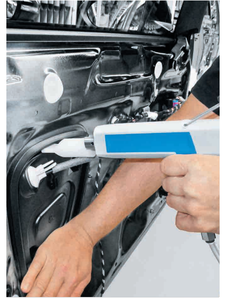
Easier automotive assembly: the clip fix tool AGTC reduces ergonomic strain on finger and hand joints.
